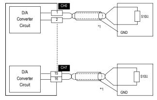
\*1 For the cable, use a two-core twisted shielded wire
