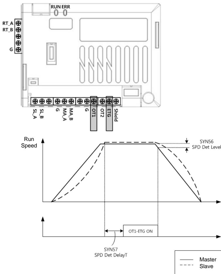
Open Collector Digital Output Contact 1 ON :
