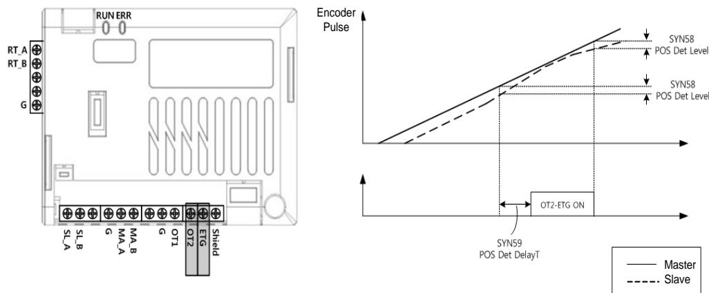
It is possible to monitor the state of Open Collector Digital Output Contact 2 from SYN-03 Sync DO Stat as seen inside of a dotted line of the following figure.
