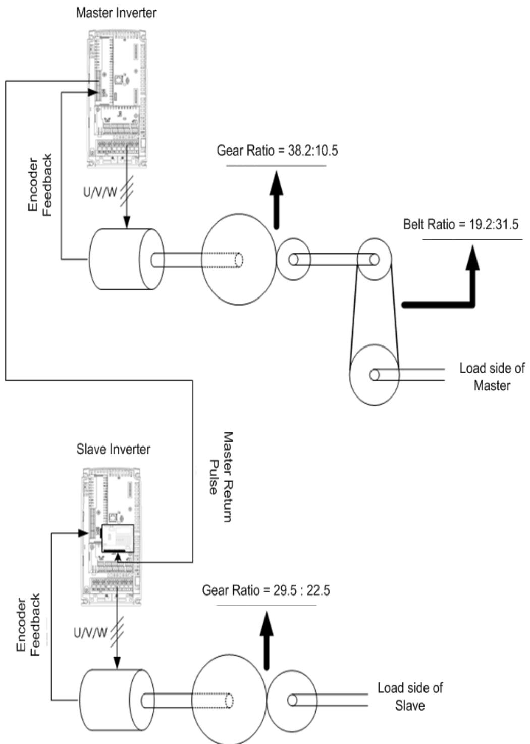
Input the gear ratio of the master/slave side respectively.
