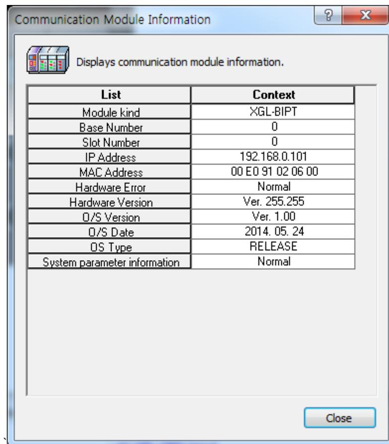
[Figure 1.4.2] Version identification of module through XG-PD
