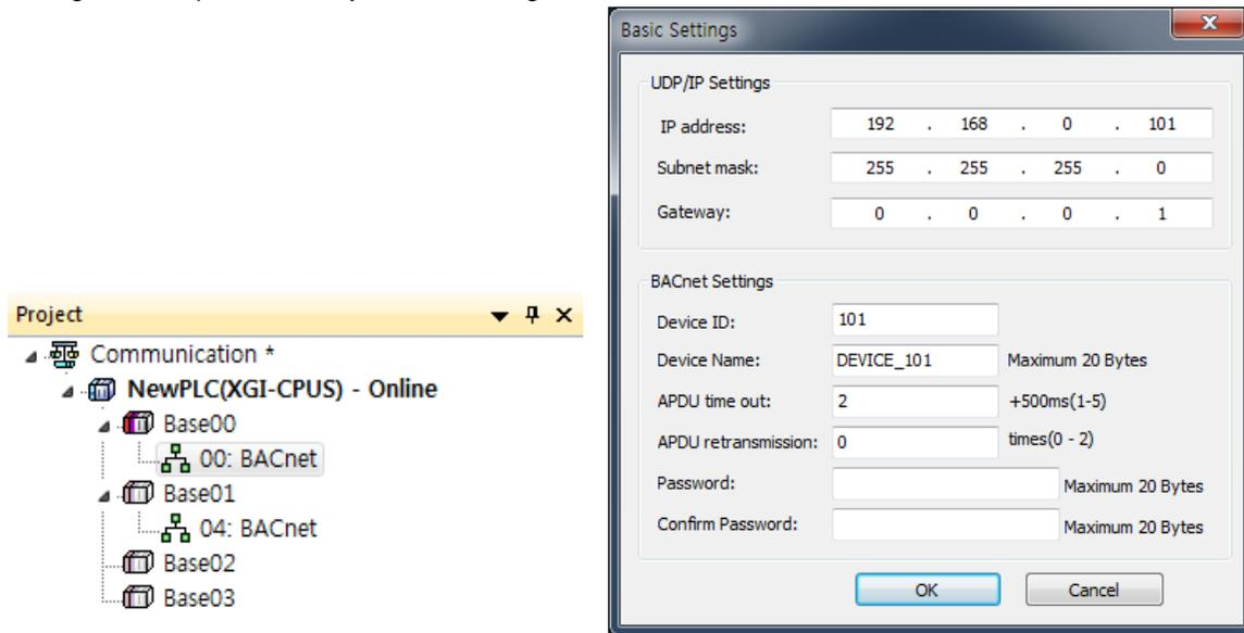
Figure 2 Basic Parameter Setting
