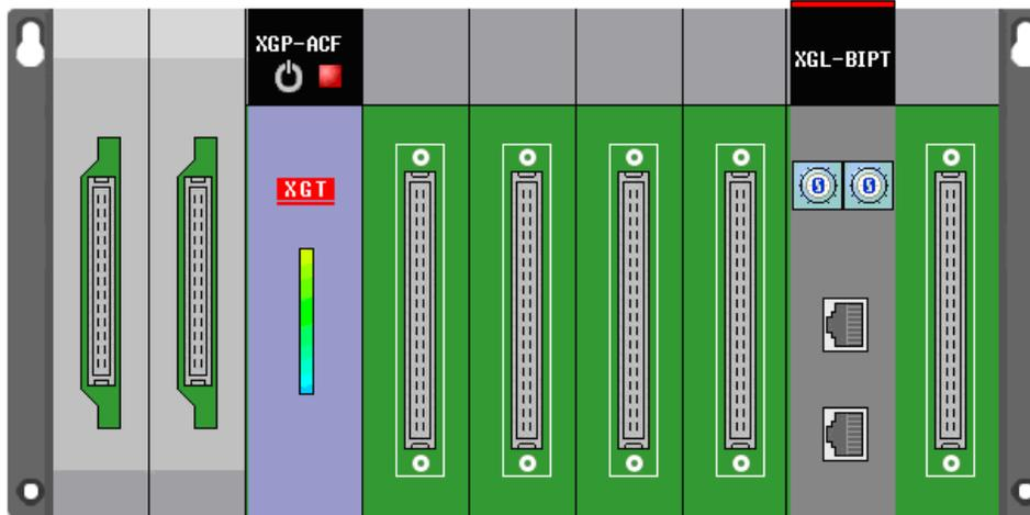
[Figure 7.1.3] System Diagnosis Screen for Augmenting base
