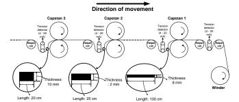
Fig. 2.7.1 Capstan operating mechanism
