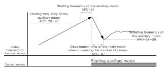
Starting sequence of the auxiliary motor by load increase
