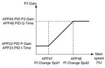
Fig. 1.5.3 Switching the PI gain depending on speed
