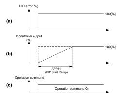
Fig. 3.3.2 Activating APP51 (PID Start Ramp)
