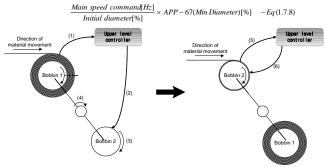
Fig. 1.7.2 Conceptual diagram of splicing
