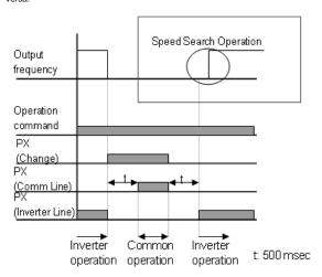
IN-55 - 75 Px Define: Sets the No.15 Exchange and switches the motor from inverter power to commercial power. Turn OFF the preset terminal to switch the motor from commercial power to the inverter output terminal.
