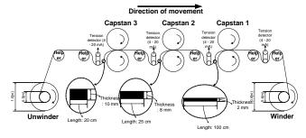
Fig. A1.1 An imaginary tension control system
