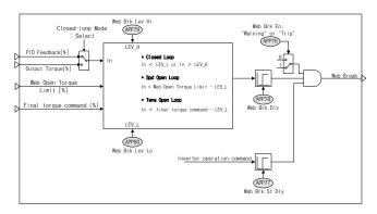
Closed loop tension control systems use tension detectors, such as the dancer or load cell. When the feedback from the tension detector is shorter or longer than the time specified, the inverter determines that the web material may be ruptured. It then informs the upper level controller of the potential risk via the multi-function output contact and initiates the proper protective operation based on this setting.
