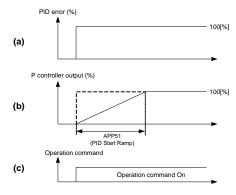
Fig. 1.5.1 Activating APP51 (PID Start Ramp)
