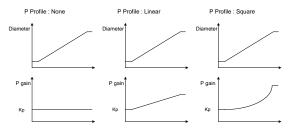
Fig. 1.5.2 The P gain trend varies depending on the APP56 settings (Profile P Mode)
