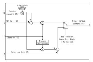
Final tension computation is available in tension control closed loop/open loop systems.
