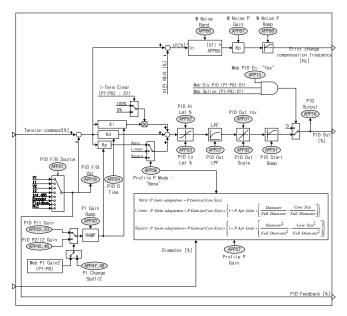
In a closed loop tension control system, the analog quantity feedback from tension detectors, such as the dancer or load cell, determine the PID controller output. A PID controller optimized for tension control systems is referred to as a Web PID controller.
