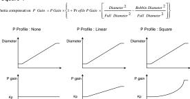
Fig. 1.5.2 The P gain varies depending on the CON90 (ASR P Pro Mode) setting
