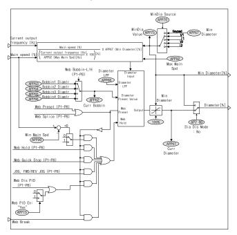
In a tension control system, the winder/unwinder flux, motor speed, and diameter are correlated, as shown in Eq. 1.6.1.
