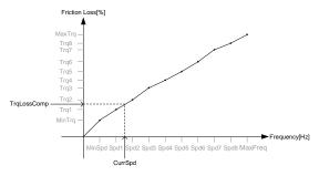
Fig. 1.11.1 Friction loss by speed
