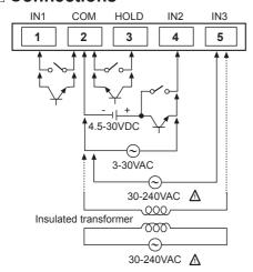
※Please use reliable contacts enough to flow 5µA of current when using input signal or reset signal as a contact.
