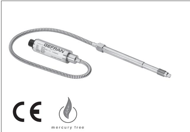
The K3 Series are for use in high temperature applications where the process temperatures may reach 538°C (1000°F) such as high temperature engineered polymers. The K Series utilizes standard melt pressure principles and construction, but uses a near incompressible NAK (Sodium Potassium) for pressure transmission. The K Series strain sensing technology is bonded foil strain gage.
