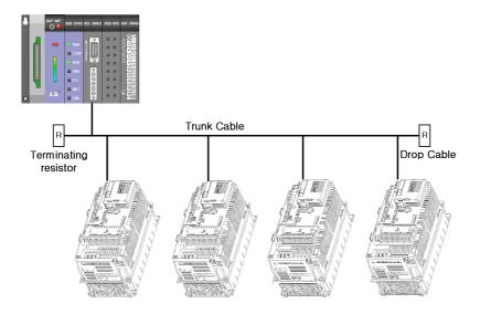
For DeviceNet communication, DeviceNet standard cable specified by ODVA should be used. There are Thick or Thin type cable as DeviceNet standard cable. For DeviceNet standard cable, refer to ODVA homepage (<a href="http://www.odva.org">http://www.odva.org</a>).
