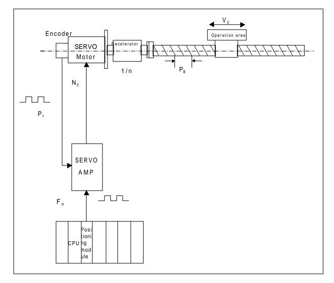
Items necessary to calculate shifting amount per pulse are supposed as described below.
