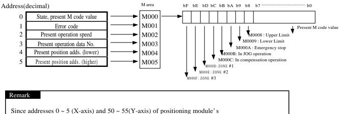
Since addresses 0 ~ 5 (X-axis) and 50 ~ 55(Y-axis) of positioning module's buffer memory are the area exclusively for Read, Read of positioning module status shall be performed by GET command.
