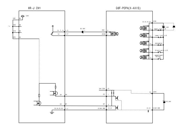
\*1 : In case that internal power is used. Refer to the driver manual for the driver pins if not described. 5) Connection with UPD566 (stepping motor driver)
