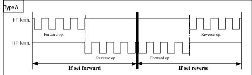
Reverse rotation : Rotation direction is set to the direction where present value of position address is
