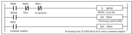
Data-accompanied command shall be processed simultaneously with data and command under the same conditions, or positioning module may be abnormal in operation.
