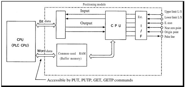
[Fig. 10.2] Structure of positioning module
