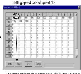
Use speed teaching when speed value "100(1Kpps)" of speed No.0 is applied as changed to new value.
