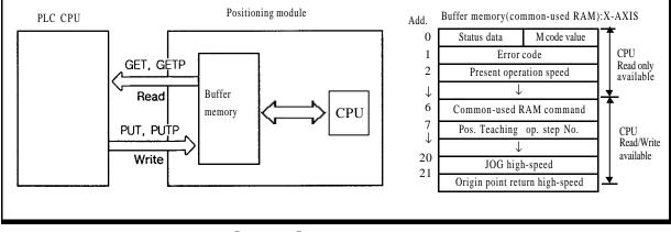
[Fig. 10.5] Buffer memory (common-used RAM)
