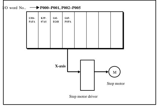
[Fig.10.1] System configuration of basic example program
