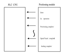
[Fig.10.3] Input signal of positioning module
