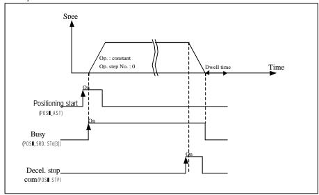
6) Positioning constant operation mode (positioning complete)
