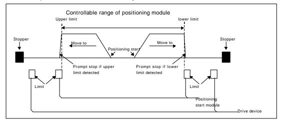
Positioning operation is not available if positioning module is stopped out of controllable range.
