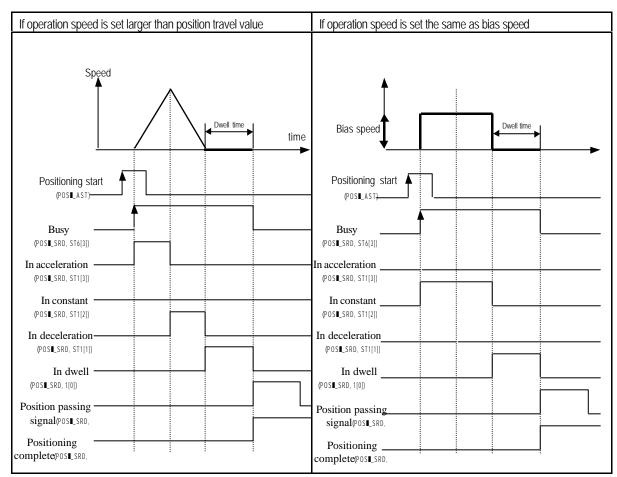
2) Repeated operation mode (positioning complete)
