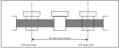
Range check of upper/lower stroke limit is performed at operation start and during operation.. If an error is detected by S/W upper/lower stroke limit value setting (S/W stroke upper limit address range exceeded : 25, S/W stroke lower limit address range exceeded : 24), pulse output of positioning module is prohibited.
