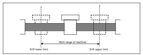
Function not to execute positioning by its applicable command if operated out of the setting range.
