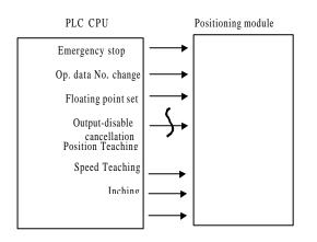
**[**Fig. 10.4**]** Output of positioning module
