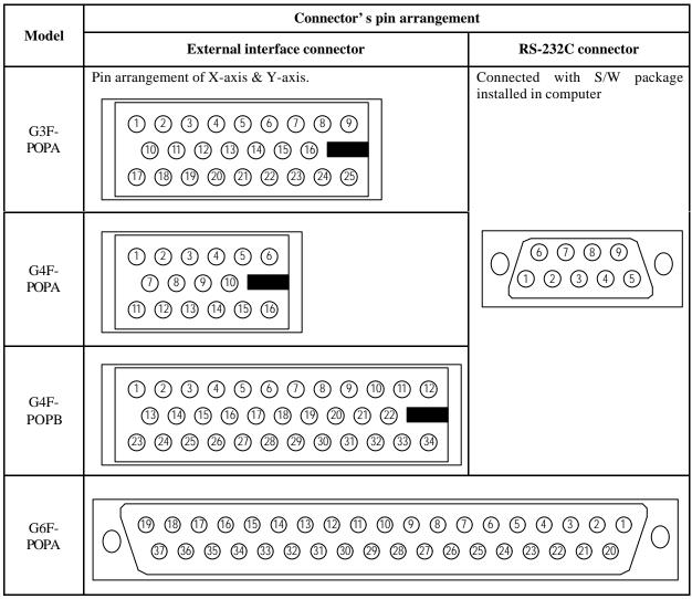
Direct connection is unavailable between G6F-POPA positioning module and computer.
