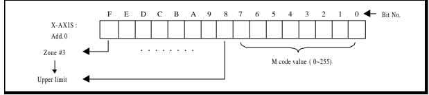
[Fig. 10.6] Example of buffer memory (common-used RAM)
