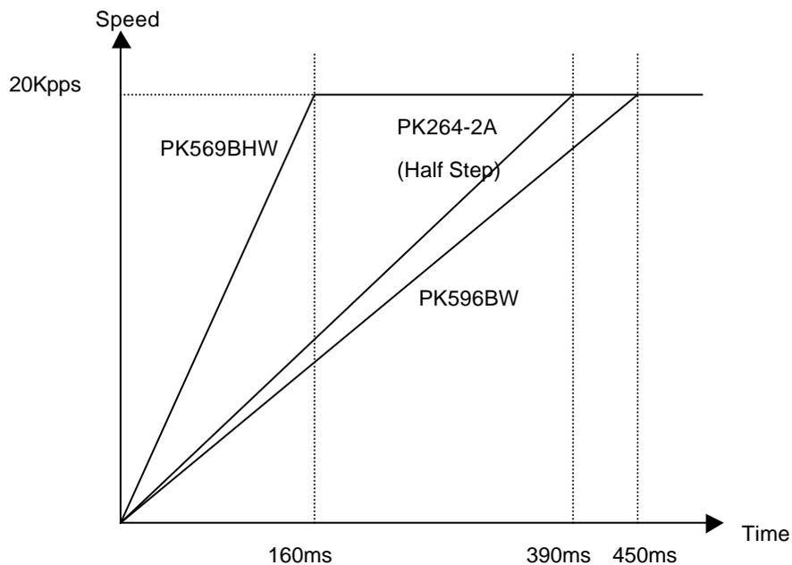
**Table1. Testing example of G6F-POPA stepping motor's max. accel./decel. inclination**
