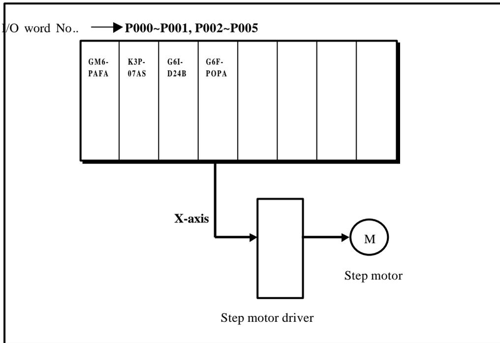
[Fig.10.1] System configuration of basic example program
