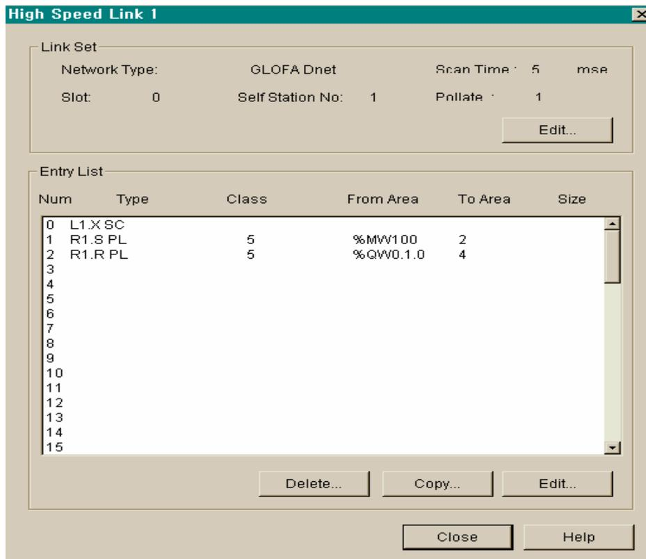
3) Setting of *high speed link* parameter on GM6 #2(station 2)
