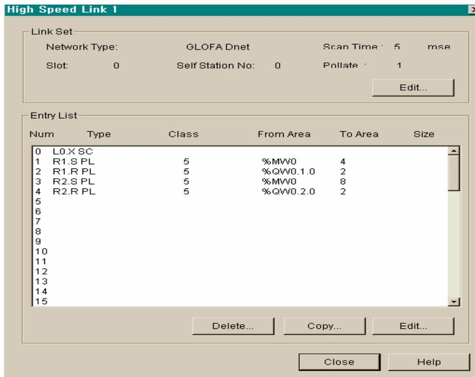
2) Setting parameter for *high speed link* on GM6 #1(station 1)
