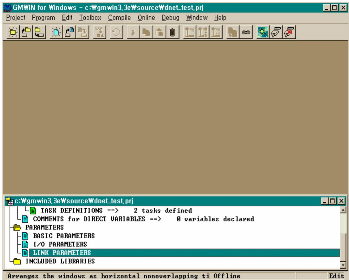
[Fig. 6.2] Display for selecting *High speed link* parameter
