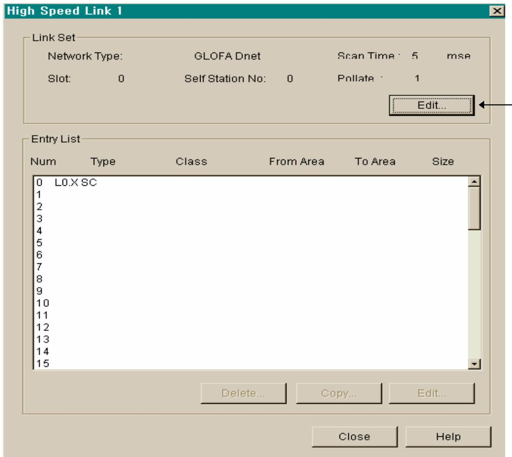
[Fig 6.4] Display for setting of *High speed link*
