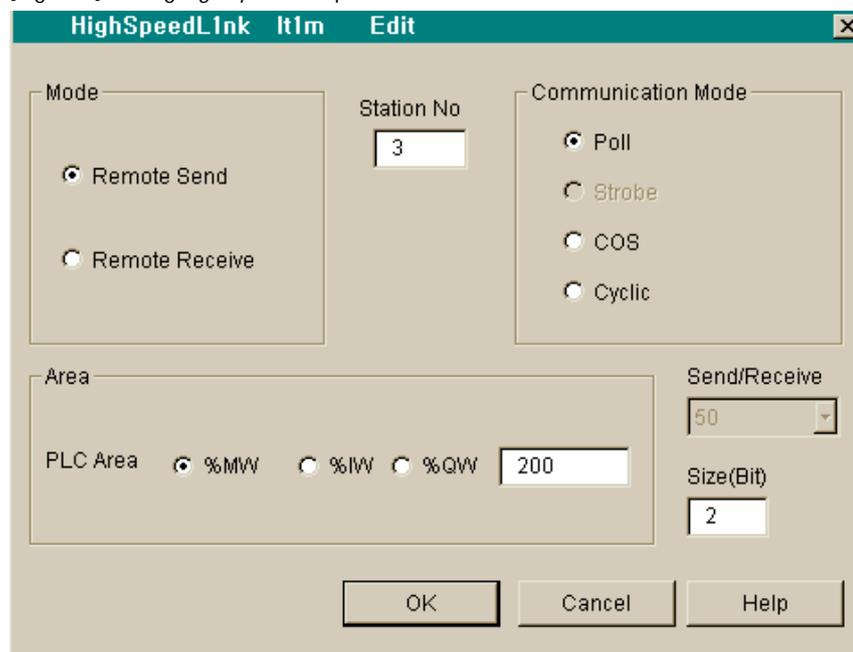
[Fig 6.13] shows setting method of sending data on single type I/F output module(G0L-DSQA). Mode among parameter sets alternative of data receiving or not, the opposite station number(G0L-DSQA), communication mode is poll, data area to be sent and the size should be set as 2. There is no additional setting on single type I/F module and it's being controlled on master module according to communication speed.
