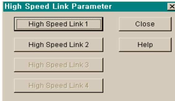
If you select '*High speed link 1*' [Fig.6.3] will be shown. And then select '→' symbol on [Fig.6.3] display to set slot position where Dnet I/F module is attached and station number, operation mode, scan time and pollate.
