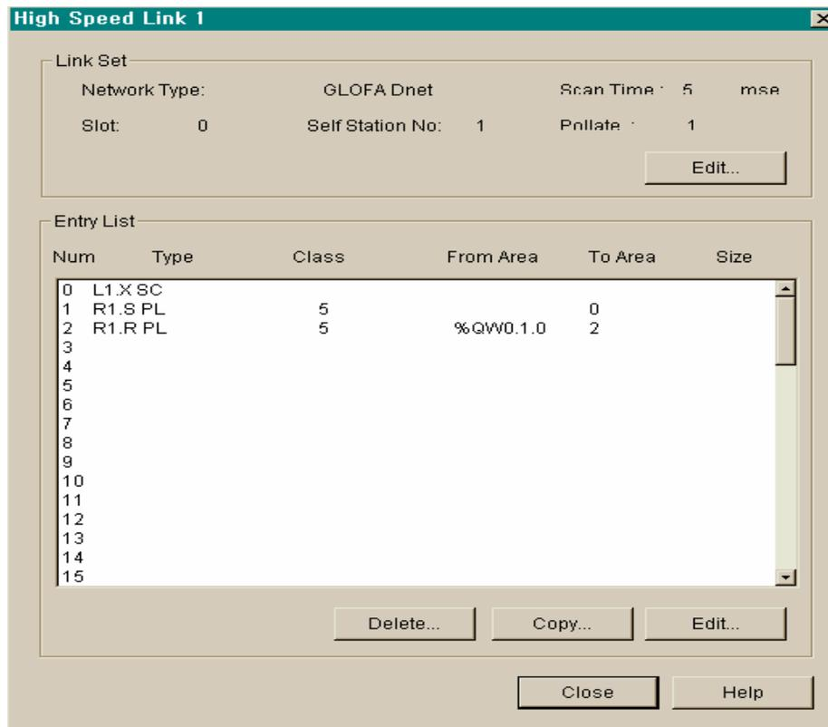
3) Setting parameter for *high speed link* on GM6 #2(station 2)
