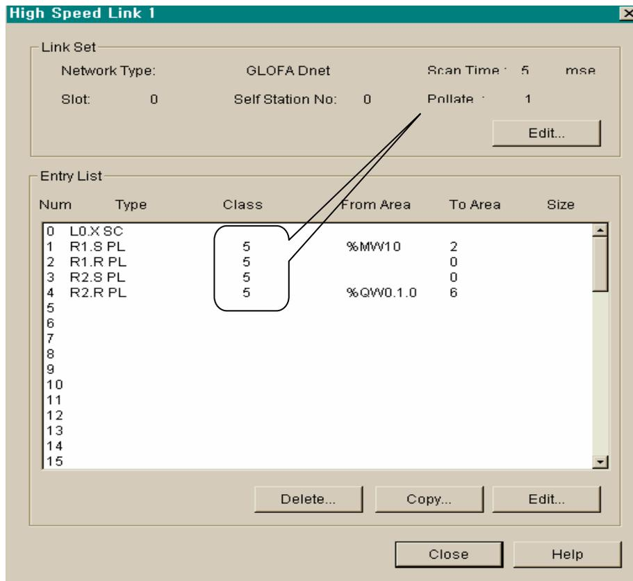
2) Setting *high speed link* parameter on GM6 #1(station 1)
