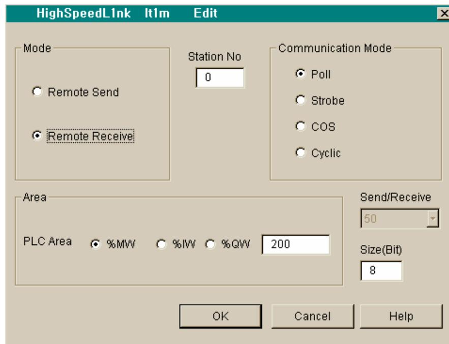
[Fig 6.12] Setting of sending parameter as slave function
